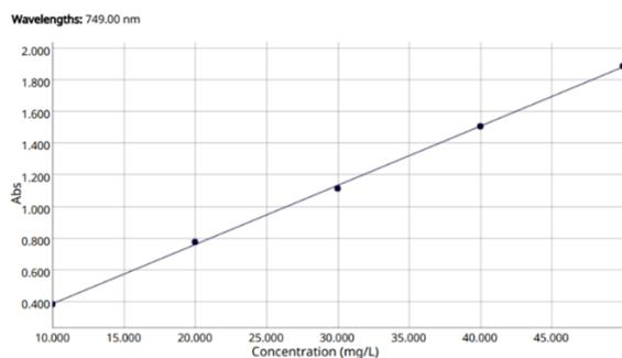
Figure 2: Graph of the Measurement Result Curve of the Absorbance Value of a Standard Solution Gallic Acid of N-Hexane Extract.
