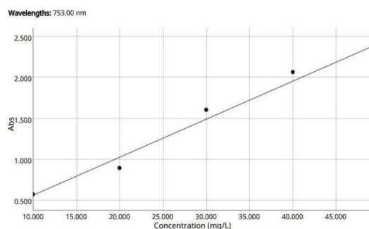
Figure 1: Graph of the Measurement Result Curve of the Absorbance Value of a Standard Solution Gallic Acid of Ethanol Extract.
